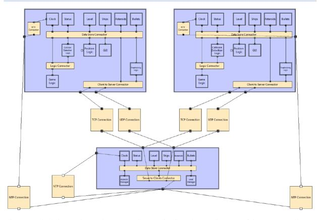
The game is divided into a client and a server application. The above diagram shows two of clients connected to a server, all of them with their internal component structure. The game architecture does not pose any explicit limits on the number of clients simultaneously connected to the game server.
