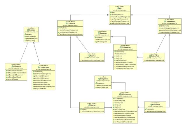
Based on this class model, I could implement the structural composition of the game components and connectors exactly and explicitly as described in the architecture models. Both client and server use the same Data Store Connector and data store components implementation, but connect different components on the bottom side of the connector. The package/class diagrams below illustrate the entities involved in the implementation.
